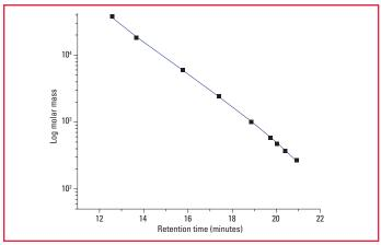
Figure 1. RI Calibration Curve for PStQuick Kit-L polystyrene standards at 0.3 mL/min in THF at 35 °C
