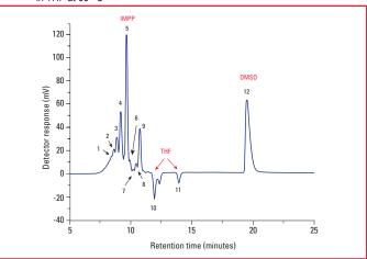
Figure 4. SEC elution profile of IMPP sample as monitored by RI (blue) at 0.6 mL/min in THF at 35 °C
