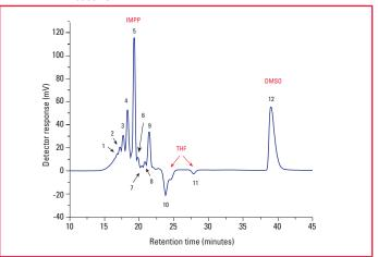
Figure 2. SEC elution profile of IMPP sample as monitored by RI (blue) at 0.3 mL/min in THF at 35 °C
